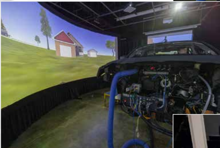
During a simulation, the driver's reaction time may be tested by a surprise event, such as a trash can rolling into the road.
