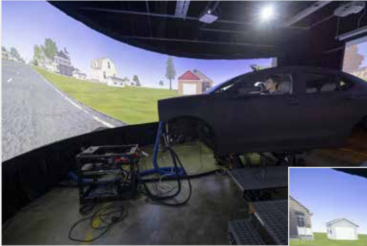
During a simulation, the driver's reaction time may be tested by a surprise event, such as a trash can rolling into the road.
