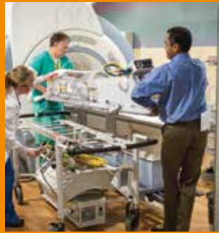
The team lifts the MRI-compatible infant incubator onto the MRI table. The 3.0 Tesla magnet is nearly twice the strength of standard clinical imaging machines.
